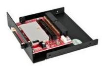
This Compact Flash IDE adapter is a perfect solution for accessing CompactFlash (CF I, CF II) and IBM Micro Drive media, allowing you to access the flash/micro drive media as if it were an IDE hard drive.
