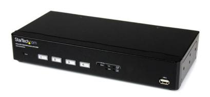
The SV431DVIUDDM 4-Port USB DVI KVM Switch lets you control 4 DVI, USB-equipped PCs using a single peripheral set at high-definition DVI resolutions up to 1920x1200.
