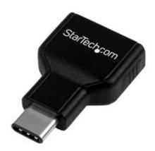
This USB-C<sup>™</sup> to USB-A adapter lets you connect standard USB 3.0 and USB 2.0 devices to your USB-C equipped phone, tablet or computer. Simply plug the adapter into the USB Type-C<sup>™</sup> port to turn it into a USB Type-A port, and you're ready to connect your older devices. The adapter is compatible with USB 3.0 enabled computers, such as the Dell<sup>™</sup> Latitude<sup>™</sup> 11 5000 2-in-1, and more.
