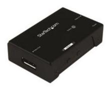
This DisplayPort signal booster lets you increase the signal strength of your DP video source using standard DisplayPort cables. You can achieve resolutions up to 4K at 60Hz, and depending on your desired resolution, the booster supports varying distances up to 65 ft. (20 m) away at 1080p 60Hz resolution. For inline installations, you can place the booster between two DisplayPort cables, up to 50 ft. in length at the video output, and up to 15 ft. in length at the video output.
