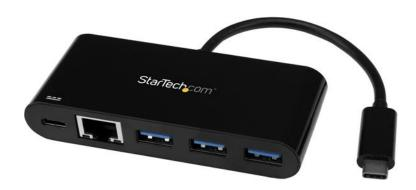
Add powerful connectivity to your USB-C enabled laptop, tablet or desktop computer. Ideal for mobile use, this USB-C to Ethernet adapter plugs into your USB-C or Thunderbolt™ 3 port to provide wired network access, and gives you three USB 3.0 Type-A ports to connect your peripheral devices. Plus you can charge your laptop as you work. It makes a great companion for your MacBook, Chromebook Pixel™, Dell™ XPS 12, or other device.
