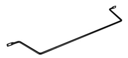
These lacing bars install horizontally on the front or back of your rack to provide a secure mounting point for you to run cables. You can attach your cables to the lacing bars using cable ties to reduce the tension on your cables and prevent damage to the ports on your rack-mount equipment. The lacing bars feature a 4 in. offset for hassle-free cable access.
