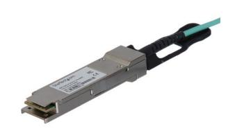
The QSFP40GAO7M is an MSA compliant optical quad small form-factor pluggable (QSFP+) cable that is designed, programmed and tested to work with 40 GbE compatible switches and routers. This AOC QSFP+ cable supports 40 Gigabit Ethernet applications (4 x 10GbE) connected through QSFP+ ports. It is a low-power, low-latency cable that is hot-swappable, making upgrades and replacements seamless by minimizing network disruptions.
