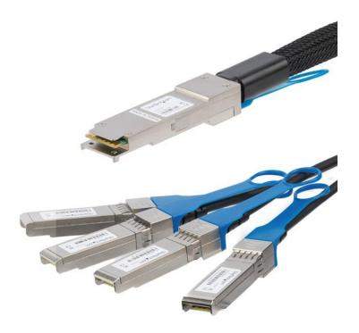
The QSFP4SFP10C5 is a Cisco QSFP-4SFP10G-CU5M compatible QSFP+ direct-attach breakout cable. It is designed, programmed and tested to work with Cisco® brand compatible servers or routers and complies with MSA industry standards. Connecting a single QSFP+ port to four 10G SFP+ ports, this passive copper breakout cable is fully hot-pluggable which makes upgrades and replacements seamless by minimizing network disruptions.
