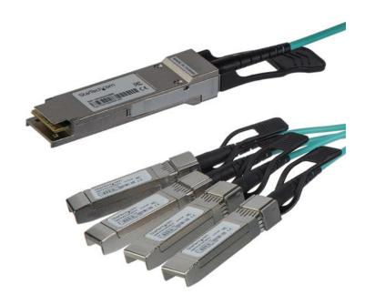
The QSFP4X10GAO7 is a Cisco QSFP-4X10G-AOC7M compatible optical quad small form-factor pluggable (QSFP+) breakout cable that is designed, programmed and tested to work with Cisco® brand compatible servers or routers and complies with MSA industry standards. Connecting a single QSFP+ port (40 GbE) to four 10G SFP+ ports, this active optical breakout cable is fully hot-pluggable which makes upgrades and replacements seamless by minimizing network disruptions.
