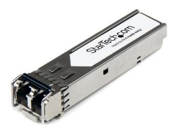
The EW3F0000710-ST is a Citrix EW3F0000710 compatible fiber transceiver module that has been designed, programmed and tested to work with Citrix brand switches and routers. It delivers dependable 10 GbE connectivity over fiber cable, for 10GBase-SR compliant networks, with a maximum distance of up to 300 m (984 ft).
