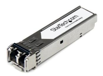
The EW3Z0000586-ST is a Citrix EW3Z0000586 compatible fiber transceiver module that has been designed, programmed and tested to work with Citrix brand switches and routers. It delivers dependable 10 GbE connectivity over fiber cable, for 10GBase-LR compliant networks, with a maximum distance of up to 10 km (6.2 mi).
