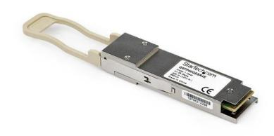
The QSFP-40G-SR4-AR-ST is an Arista Networks QSFP-40G-SR4 compatible fiber transceiver module that has been designed, programmed and tested to work with Arista Networks brand switches and routers. It delivers dependable 40 GbE connectivity over fiber cable, for 40GBase-SR4 compliant networks, with a maximum distance of up to 150 m (492 ft).
