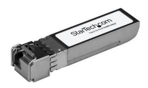
The SFP-10G-BX-D-40-ST is a Cisco SFP-10G-BX-D-40 compatible downstream fiber SFP transceiver which pairs with StarTech.com's SFP-10G-BX-U-40-ST. They are designed, programmed and tested to work with 10GBase-BX compatible Cisco switches and routers. The SFP+ transceiver module supports a maximum distance of up to 40 km (24.8 mi) and delivers dependable 10 GbE connectivity over fiber cabling.
