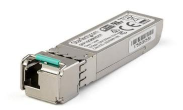
The SFP10GBX40US is a Dell EMC SFP-10G-BX40-U compatible upstream fiber SFP transceiver which pairs with StarTech.com's SFP10GBX40DS. They are designed, programmed and tested to work with 10GBase-BX40 compatible Dell EMC switches and routers. The SFP+ transceiver module supports a maximum distance of up to 40 km (24.8 mi) and delivers dependable 10 GbE connectivity over fiber cabling.
