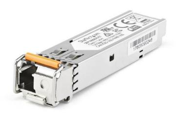
The SFP1GBX40UES is a Dell EMC SFP-1G-BX40-U compatible upstream fiber SFP transceiver which pairs with StarTech.com's SFP1GBX40DES. They are designed, programmed and tested to work with 1000Base-BX40 compatible Dell EMC switches and routers. The SFP transceiver module supports a maximum distance of up to 40 km (24.8 mi) and delivers dependable 1 GbE connectivity over fiber cabling.
