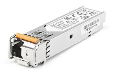
The SFP1GBX80UES is a Dell EMC SFP-1G-BX80-U compatible upstream fiber SFP transceiver which pairs with StarTech.com's SFP1GBX80DES. They are designed, programmed and tested to work with 1000Base-BX80 compatible Dell EMC switches and routers. The SFP transceiver module supports a maximum distance of up to 80 km (49.7 mi) and delivers dependable 1 GbE connectivity over fiber cabling.
