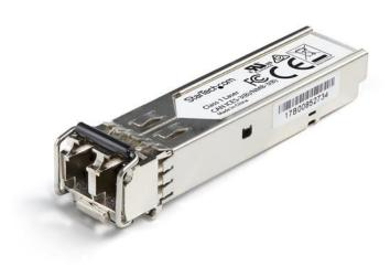
The SFP1GLXEMCST is a Dell EMC SFP-1G-LX compatible fiber transceiver module that has been designed, programmed and tested to work with Dell EMC brand switches and routers. It delivers dependable 1 GbE connectivity over fiber cable, for 1000Base-LX compliant networks, with a maximum distance of up to 10 km (6.2 mi).
