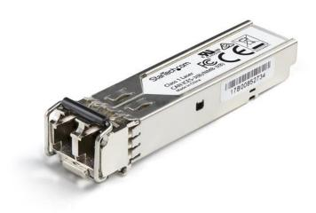
The SFP1GSXEMCST is a Dell EMC SFP-1G-SX compatible fiber transceiver module that has been designed, programmed and tested to work with Dell EMC brand switches and routers. It delivers dependable 1 GbE connectivity over fiber cable, for 1000Base-SX compliant networks, with a maximum distance of up to 500 m (1640 ft)).
