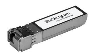
The 10G-SFPP-BXD-40K-ST is a Brocade 10G-SFPP-BXD-40K compatible downstream fiber SFP transceiver which pairs with StarTech.com's 10G-SFPP-BXU-40K-ST. They are designed, programmed and tested to work with 10GBase-BX compatible Brocade switches and routers. The SFP+ transceiver module supports a maximum distance of up to 40 km (24.8 mi) and delivers dependable 10 GbE connectivity over fiber cabling.
