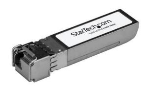
The SFP-10GB-BX-D-STA-ST is a MSA compliant downstream fiber SFP+ transceiver which pairs with StarTech.com's SFP-10GB-BX-U-STA-ST. They are designed, programmed and tested to work with 10GBase-BX compatible MSA switches and routers. The SFP+ transceiver module supports a maximum distance of up to 10 km (6.2 mi) and delivers dependable 10 GbE connectivity over fiber cabling.
